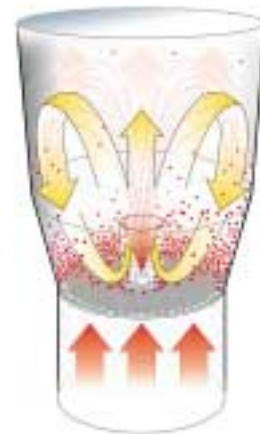
principle of bottom spray coating, Wurster
