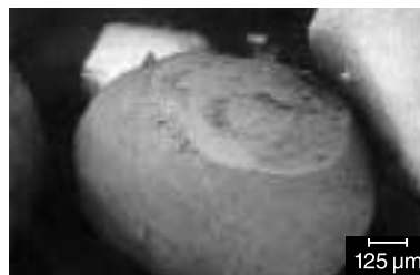
detergent component - ideal spray granule
