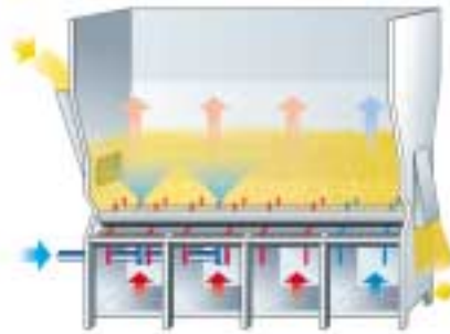
principle of continuous coating process, ProCell
